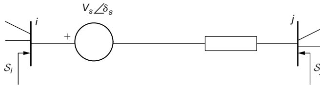
FIGURE 3.4 Voltage source model of a series compensator buses between i and j .
