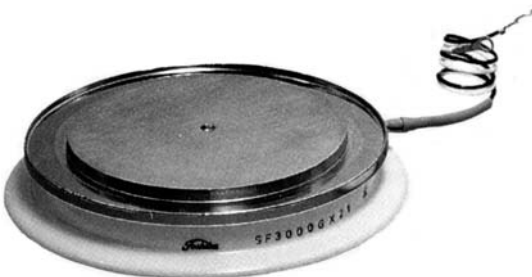
FIGURE 7.89 Commercial thyristor of the SF3000GX21 type (Toshiba) with switched current up to 3000 A (surge current is 60.000 A) and switched voltage up to 4000 V. (From Toshiba Commercial Thyristor online catalog 2004.)
