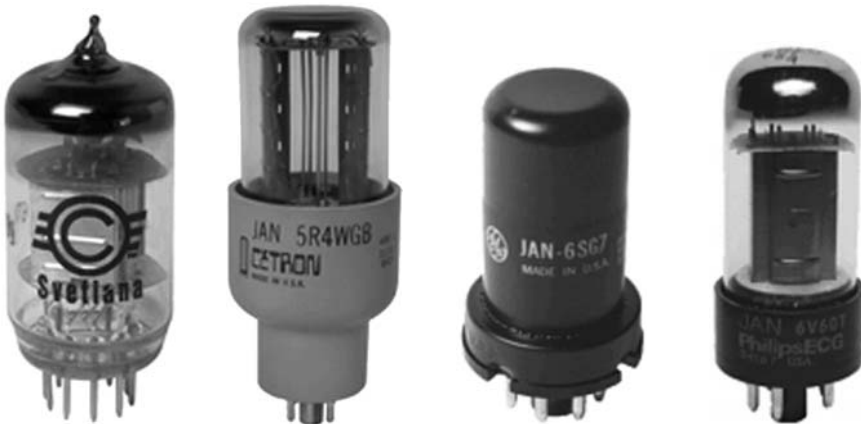
FIGURE 7.13 Modern vacuum radio valves in glass and metallic tubes, produced up to now in many countries.
