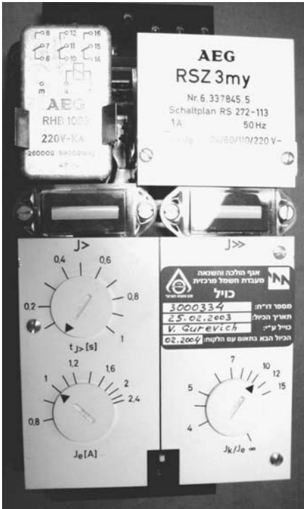
FIGURE 10.69 Fully electronic current relay, with an integrated TD element of the RSZ 3my type (AEG). Front panel view. To the left above — output electromagnetic relay. J> and J>> equal I> and I>> , respectively; t_{J>} (s) = scale of TD in seconds; J_e (A) = scale of pick-up currents in amperes (for the unit I> ); J_k/J_e = ratio of the pick-up current (for the unit I>> ).
