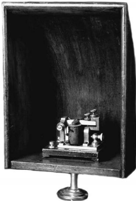
FIGURE 1.14 (a) Sounder supplied with a big wooden resonator. (b) Operator at work on telegraph key. On the rear plan a visible sounder with wooden resonator can be seen, standing on the table.
