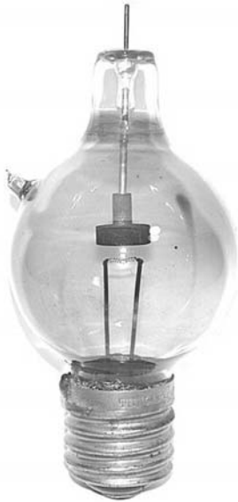
FIGURE 7.5 One of the first constructions of vacuum diodes of increased power (for current up to 6 A) based on the incandescent lamp.
