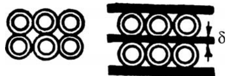
FIGURE 2.38 Laying of winding wire without spacers and with a dielectric spacer of thickness \delta between layers.
