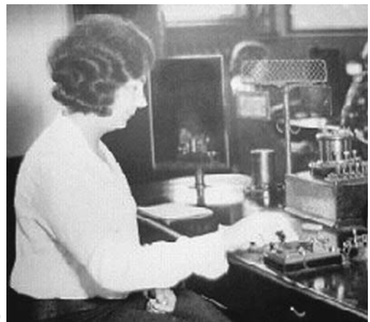
FIGURE 1.14 (a) Sounder supplied with a big wooden resonator. (b) Operator at work on telegraph key. On the rear plan a visible sounder with wooden resonator can be seen, standing on the table.
