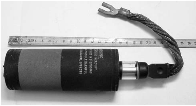
FIGURE 7.25 External design of an ignitron of the GL-5550-1 type, without additional cooling, in a metal case (General Electric Co.).
