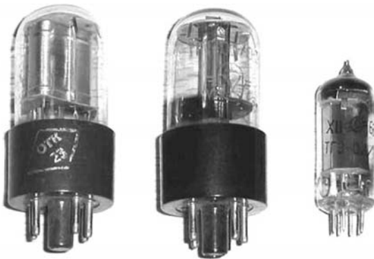
FIGURE 7.19 Low-power thyatrones with an incandescent cathode, produced in Russia.
