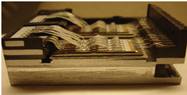
Figure 11.3 Views of boost and inverter silicon for the 2010 Toyota Prius [1]. (Courtesy of Oak Ridge National Laboratory, US Dept. of Energy.)
