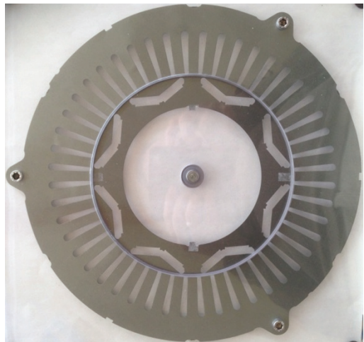
Figure 10.4 2004 Toyota Prius traction motor stator and rotor iron laminations.
