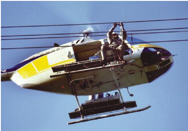
FIGURE 9.11 Working on a power line using a helicopter. (Image courtesy of USA Airmobile, Inc., Davie, FL.)
