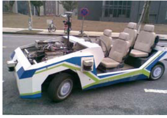
Fig. 3. The test vehicle with four in-wheel-motors
