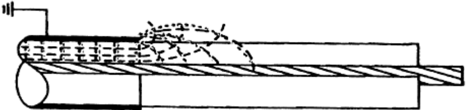
Figure 12-2 Electrical stress field with shield removed.
