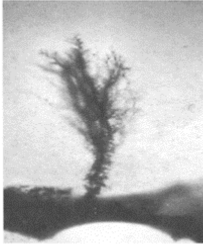
Figure 18-8 Electrical tree growing from a contaminant on conductor shield.
