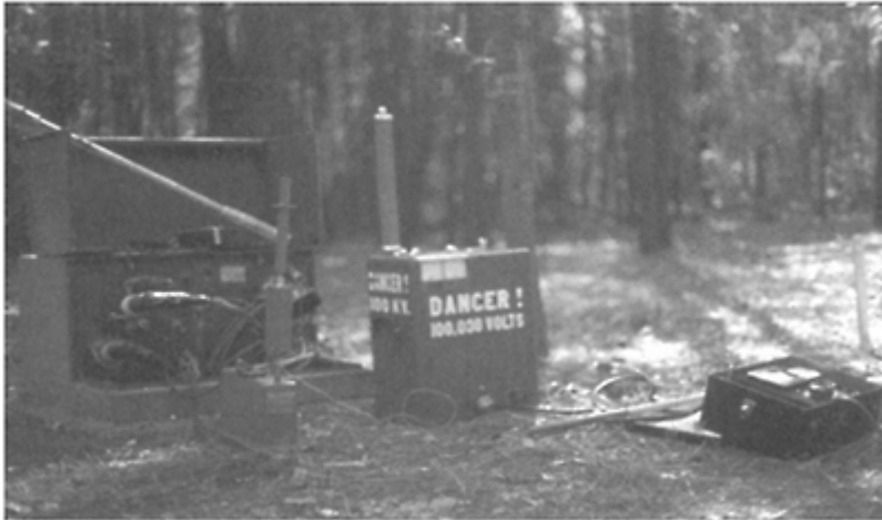
Figure 16-2 Capacitor discharge setup using non-shielded test equipment. (Photograph courtesy of Von Corporation.)
