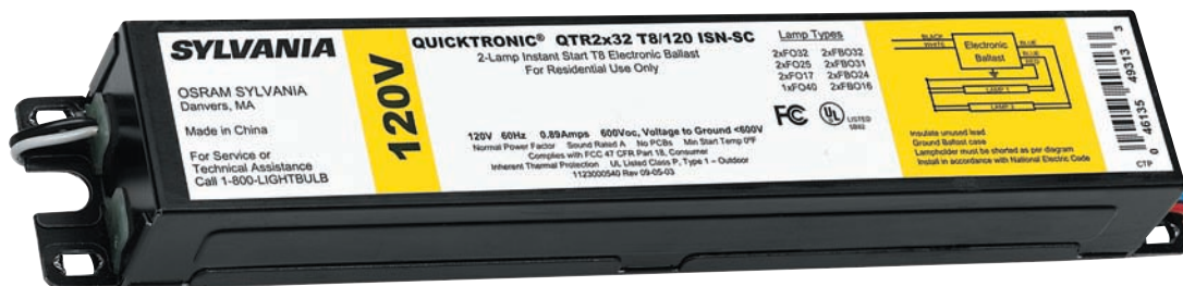
FIGURE 7-13 An electronic Class P ballast, thermally protected as required in 410.130(E). Electronic ballasts provide improved performance in fluorescent lighting installations. Electronic ballast lighting systems are 25% to 40% more energy efficient than conventional magnetic (core & coil) ballast fluorescent systems. (Courtesy of OSRAM Sylvania)
