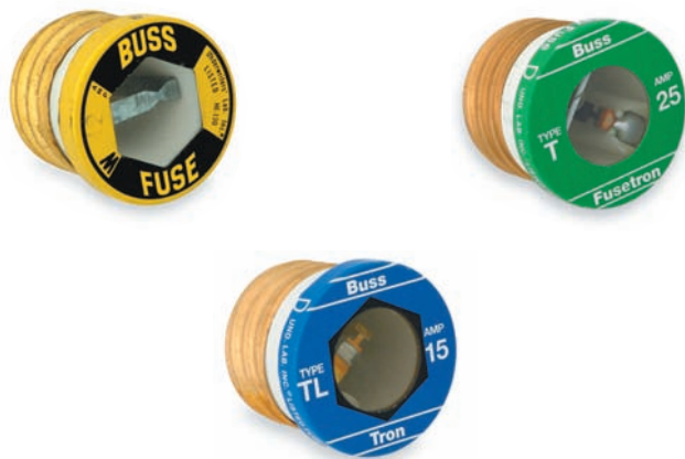
FIGURE 28-7 Three types of plug fuses: single-element, nontime-delay (W); dual-element, time-delay (T); loaded link, time-delay (TL). (Courtesy of Cooper Bussmann)
