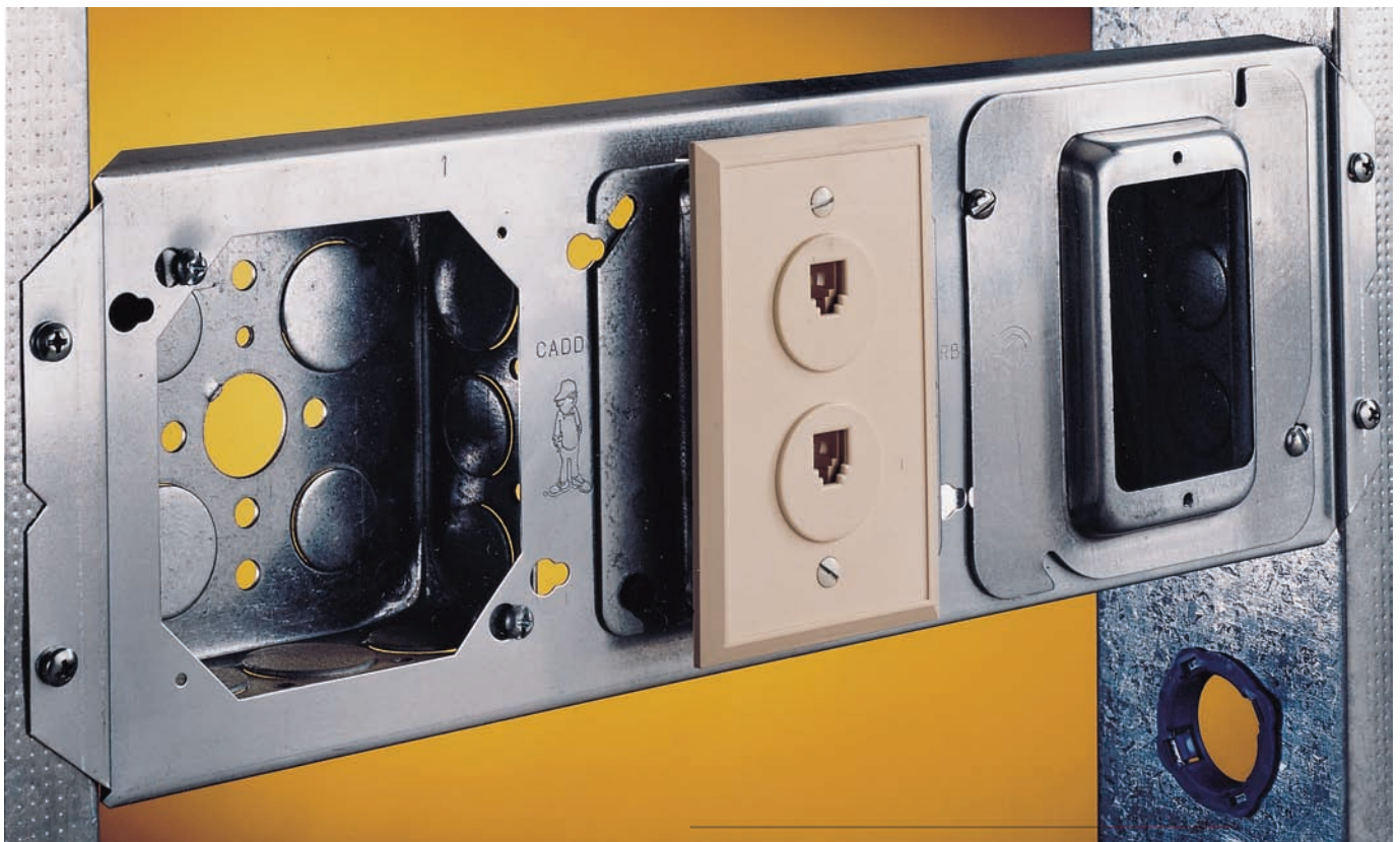
FIGURE 2-25 A bracket for use on steel framing members. The bracket spans the space between two studs. Note that more than one box can be mounted on this bracket. (Courtesy of ERICO, Inc.)
