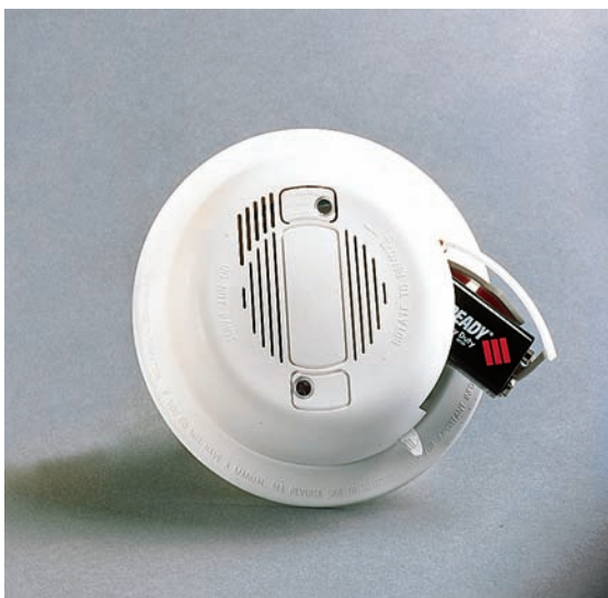
FIGURE 26-3 An ac-dc smoke alarm that operates on 120 volts ac as the primary source of power and a 9-volt battery as the secondary source of power. In the event of a power outage, the alarm continues to operate on the battery. (Courtesy of BRK Electronics)
