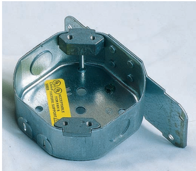
FIGURE 9-8 A special outlet box for the support of a luminaire or a ceiling-suspended (paddle) fan. There are no ears on the box. Instead, special strong mounting brackets are provided. Note that the mounting holes on the brackets are of two sizes: one set of holes is tapped for No. 8-32 screws (for a luminaire), and the other set of holes is tapped for No. 10-32 screws (for a ceiling-suspended [paddle] fan). (Courtesy of Legrand/Pass & Seymour)
