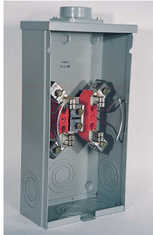
FIGURE 27-15 Typical residential self-contained meter socket. Combination meter socket/main breaker in one enclosure is also available. (Courtesy of Schneider Electric)
