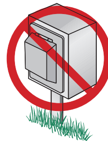
FIGURE 16-6 Raceway-supported enclosures with and without devices, 314.23(E) and (F). (Delmar/Cengage Learning)
