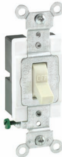
FIGURE 5-32 Single-pole toggle switch. Note that this switch has a terminal for the connection of an equipment ground conductor. Thus, when a metal face plate is installed, it will be grounded. See 404.9(A) and (B) . (Courtesy of Legrand/Pass & Seymour)
