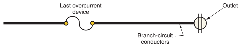
FIGURE 3-1 The branch circuit is that part of the wiring that runs from the final overcurrent device to the outlet. The rating of the overcurrent device, not the conductor size, determines the rating of the branch circuit. (Delmar/Cengage Learning)
