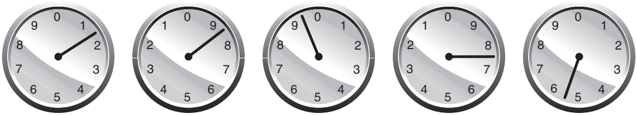
FIGURE 29-4 One month later, the meter reads 18,975 kilowatt-hours, indicating that 303 kilowatt-hours were used during the month. (Delmar/Cengage Learning)
