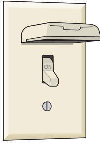
FIGURE 5-9 Switch is protected by a weatherproof cover. (Delmar/Cengage Learning)
