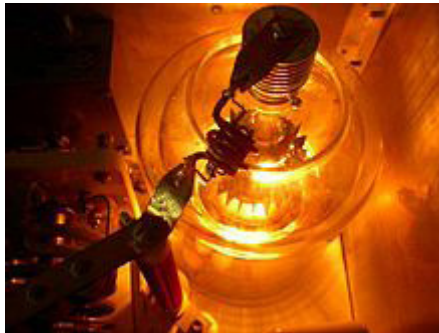
Glow from the directly heated cathode of a 1 kW power tetrode tube in a radio transmitter. The cathode filament is not directly visible
