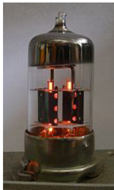
Two indirectly-heated cathodes (orange heater strip) in ECC83 dual triode tube
