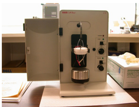
A modern cell stand for electrochemical research. The electrodes attach to high-quality metallic wires, and the stand is attached to a potentiostat/galvanostat (not pictured). A shot glass-shaped container is aerated with a noble gas and sealed with the Teflon block.
