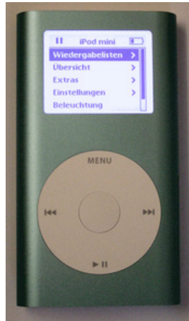
Colored iPod Mini cases are dyed following anodizing and before thermal sealing
