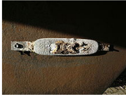
Sacrificial anode on the hull of a ship.
