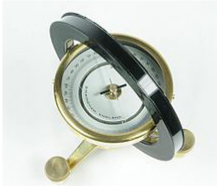
Top view of a tangent galvanometer made about 1950. The indicator needle of the compass is perpendicular to the shorter, black magnetic needle.
