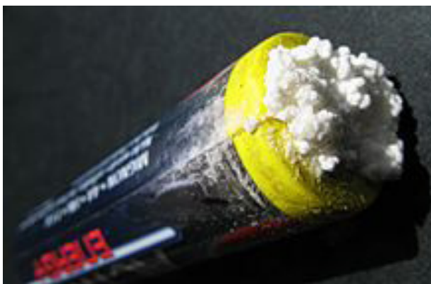
Leak-damaged alkaline battery
