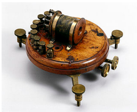
Thomson mirror galvanometer, patented in 1858.
