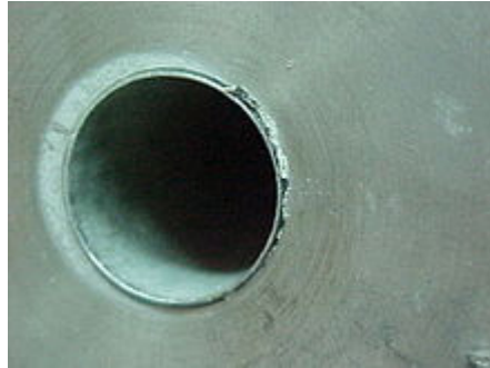
Crevice corrosion of type 316 stainless steel
