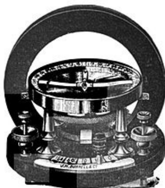
Tangent galvanometer made by J. H. Bunnell Co. around 1890.
