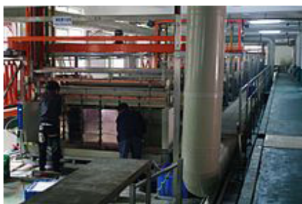
Copper electroplating machine for layering PCBs
