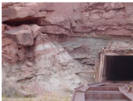
Mi Vida uranium mine, near Moab, Utah. The alternating red and white/green bands of sandstone correspond to oxidized and reduced conditions in groundwater redox chemistry.
