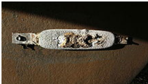
Galvanic sacrificial anode attached to the hull of a ship, showing corrosion.
