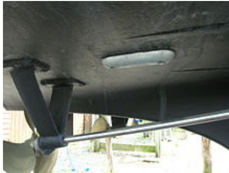
Zinc sacrificial anode ( rounded object ) screwed to the underside of the hull of a small boat.
