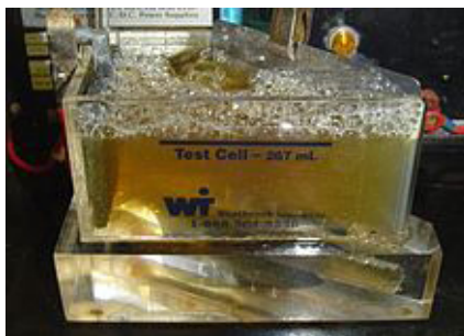
A zinc solution tested in a hull cell
