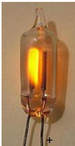
Cold cathode ( lefthand electrode ) in neon lamp
