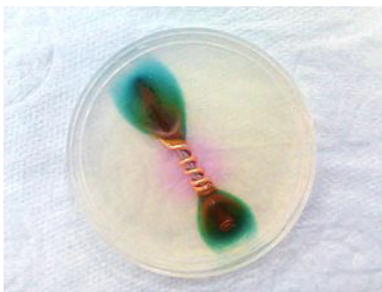
Corrosion of an iron nail wrapped in bright copper wire, showing cathodic protection of copper; a ferroxyl indicator solution shows colored chemical indications of two types of ions diffusing through a moist agar medium
