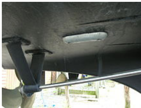
Zinc sacrificial anode (photo center) to protect a boat
