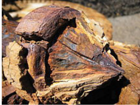
Volcanic gases have accelerated the corrosion of this abandoned mining machinery.
