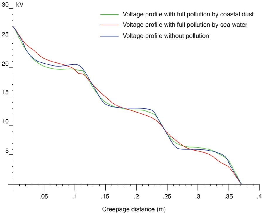
**Fig. 4.5** Voltage distribution of a line-post insulator
