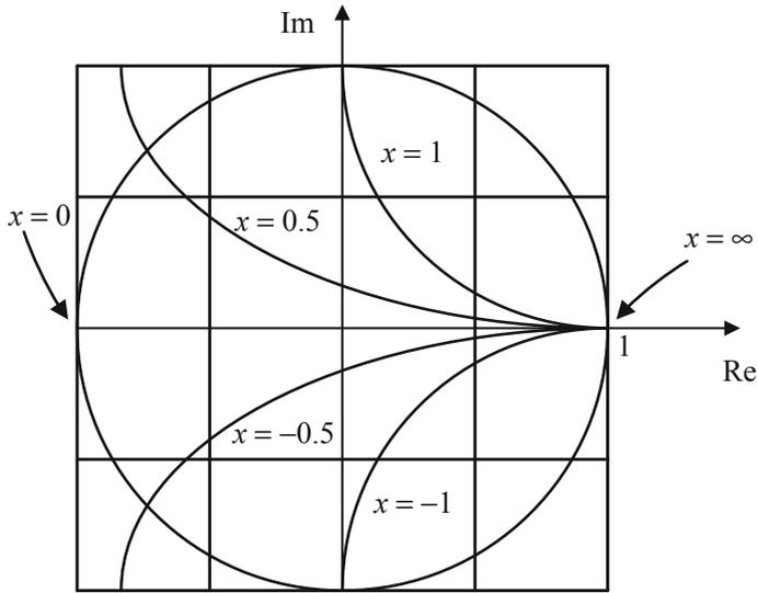
Fig. 8.9 Constant reactance circles with different radius
