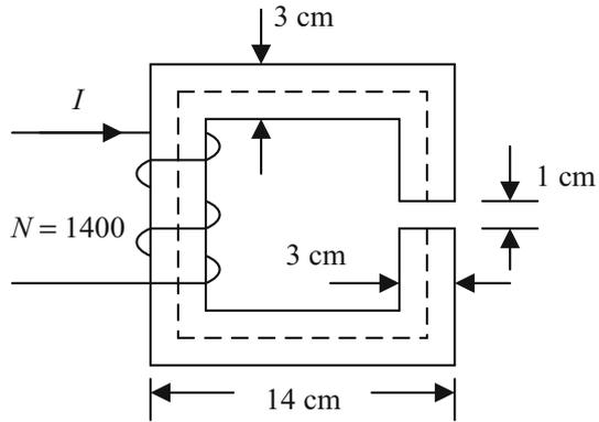
**Fig. 6.25** Magnetic circuit with a small air gap
