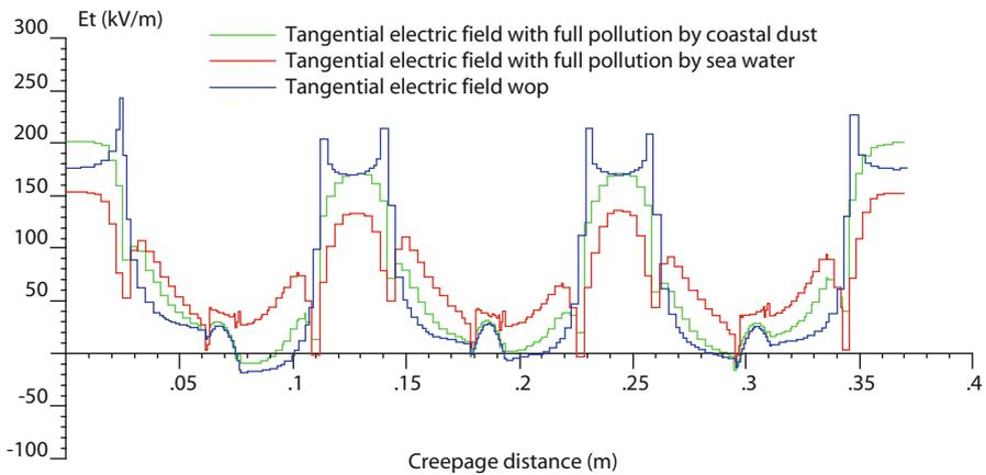
**Fig. 4.8** Tangential electric field shed–air interface of line-post insulator
