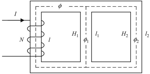
**Fig. 6.18** Equivalent parallel magnetic circuit
