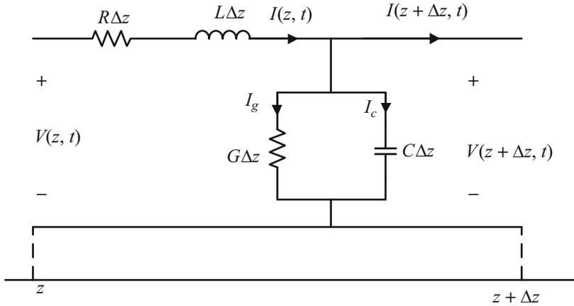
**Fig. 8.2** Equivalent circuit of a transmission line with differential length
