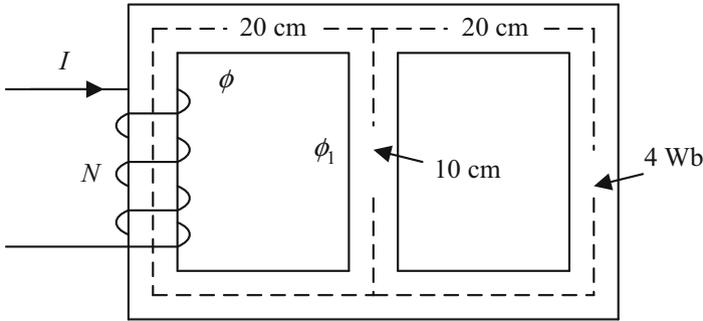
**Fig. 6.19** Parallel magnetic circuit
