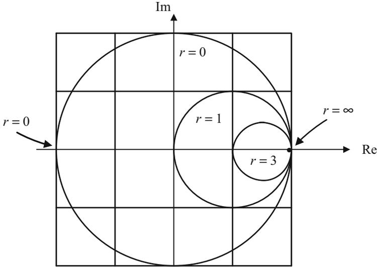
**Fig. 8.8** Constant resistance circles with different radius
