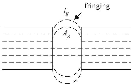
**Fig. 6.21** Magnetic circuit with an air gap
