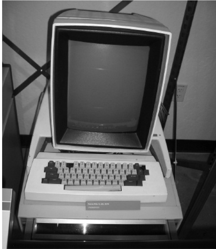
Figure 6.16 Utilitarian but revolutionary: the Xerox Alto desk computer, released in 1973, was the first nearly complete embodiment of the basic features characteristic of all later PCs (Wikimedia photograph).
