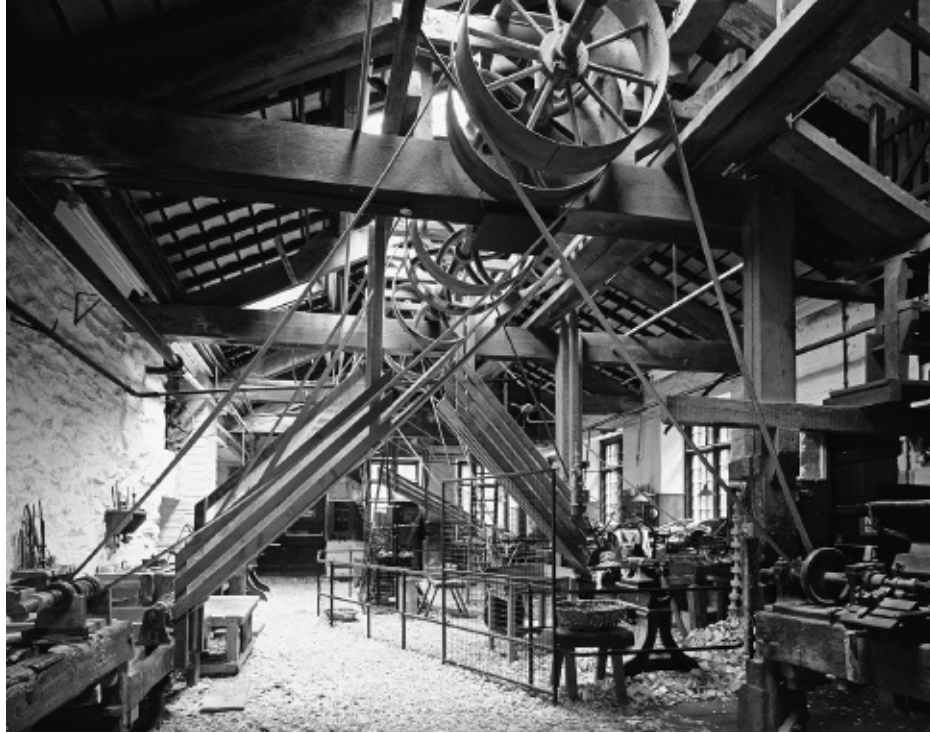
Figure 6.8 Interior of the main lathe workshop of the Stott Park Bobbin Mill in Fonthwaite, Lakeside, Cumbria, showing the typical arrangement of overhead belts transmitting power from a large steam engine to individual machines. The mill produced wooden bobbins used by Lancashire's spinning and weaving industries (Corbis).
