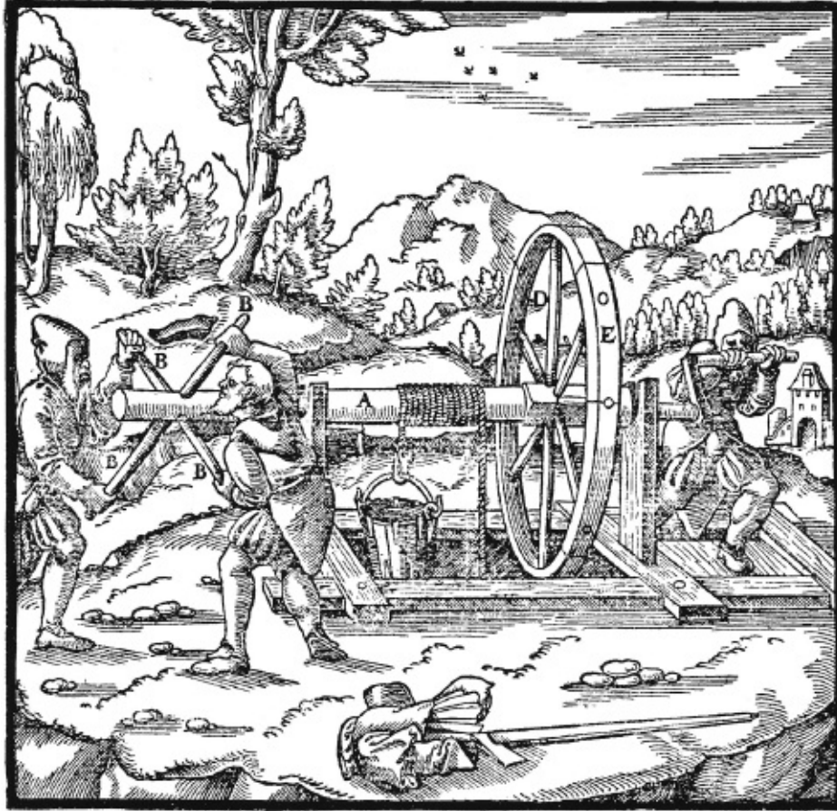
Figure 4.4 Miners using both a horizontal windlass (left) and a crank (right) to lift water from a shaft. A heavy wooden wheel, sometimes with pieces of lead fastened to its spokes, helped to conserve the momentum and make the lifting easier. Reproduced from Agricola, De re metallica (1912 [1556]).
