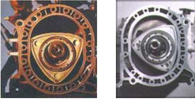
Figure I.5.3. Rotors, shaft, compartment, and the engine block of a rotary engine
