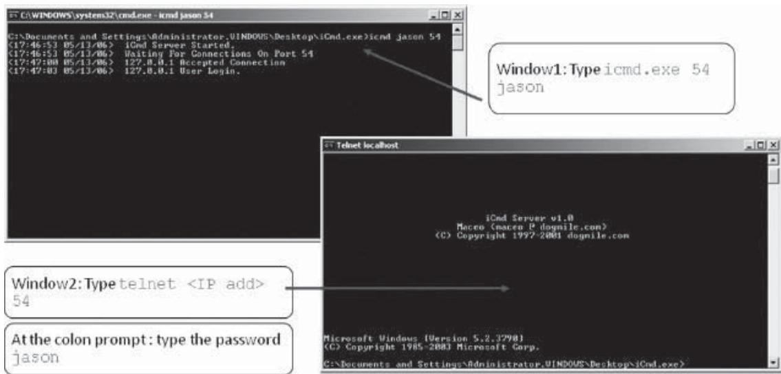
Figure 1-7 The icmd tool allows an attacker to set a password for the backdoor.
