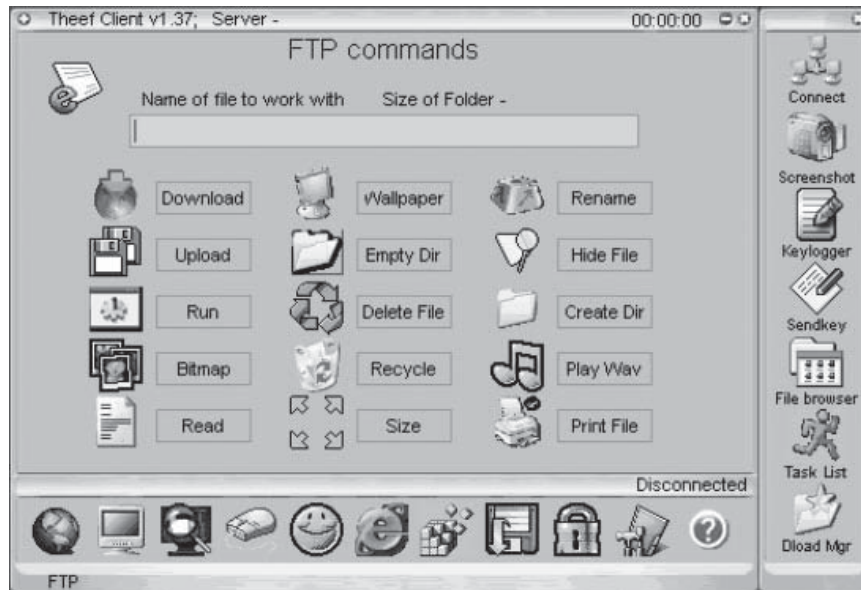
Figure 1-29 Backdoor.Theef allows attackers to perform many different functions on a victim's machine.
