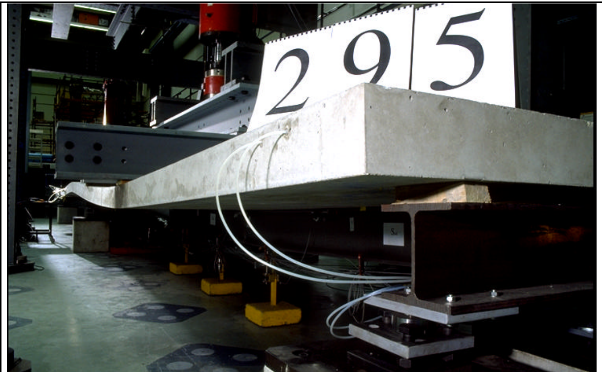
Figure 8.8. Mixed steel-concrete slab. The fiber sensors exiting concrete are visible in the foreground. The usefulness of the SOFO sensors outside the elastic domain of the structure is clearly demonstrated by this picture.
