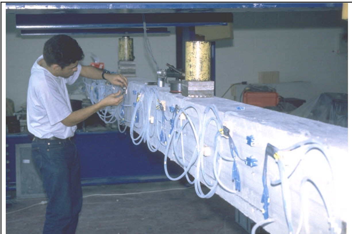
Figure 8.13. BPR concrete beam subdivided in six measurement cells each equipped with two fiber optic sensors. One near the top of the beam and the other near the bottom .
