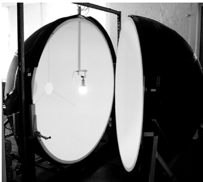
FIGURE 57.20 Photograph of an integrating sphere. Source: Reproduced with permission of the Lighting Research Center.
