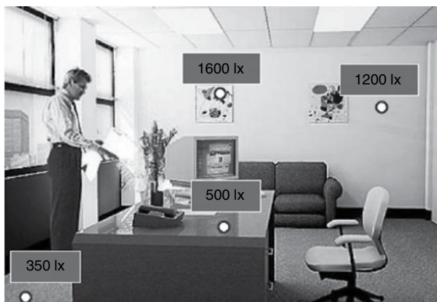
FIGURE 57.12 Distribution of selected illuminances on various surfaces within a space. Source: Reproduced with permission of the Lighting Research Center.
