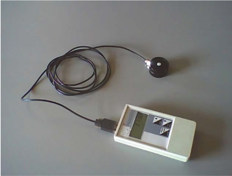
FIGURE 57.29 A portable illuminance meter with a detachable sensor element.
