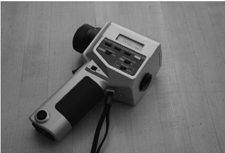
FIGURE 57.30 Portable luminance meter. Source: Reproduced with permission of the Lighting Research Center.
