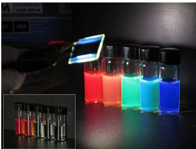
FIGURE 72.29 Depending on their size, colloidal quantum dots dispersed in hexane emit light across the entire visible spectrum (wavelengths 430–620 nm) when viewed under UV light. The inset image shows the QDs illuminated by the tungsten room light without UV irradiation. Source: Kwak et al. [203]. Reproduced with permission of the American Chemical Society.
