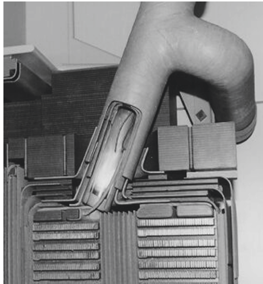
Figure 7.1.3-7: Connection of a 220 kV Lead exit system of concentric barriers to the windings of an autotransformer, cf. Figure 7.1.3-4b. Foto of the cut-away model: Weidmann, Rapperswil (CH).
