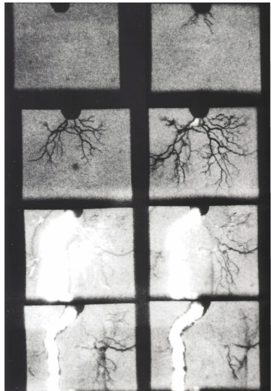
Figure 3.4.1-9: Negative discharge channels (so-called primary streamers) with branched structure [424]. For explanations see Figure 3.4.1-7.
