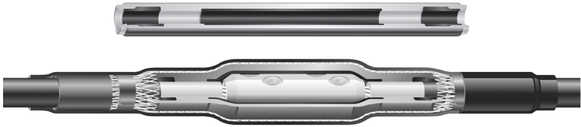
Figure 7.1.1-6: Permanent elastic connecting joint of silicone elastomer for XLPE medium voltage cables. Top: Joint body with conductive deflectors for geometric field grading (left and right, earth potential) and with "Faraday cage" for covering the metallic through connector (center, high voltage potential). Bottom: Joint mounted according to cold-shrinking technique, cf. Figure 7.1.1-7. The sheath is connected on both sides by coil springs, the outermost layer is formed by the external tube. Photos Tyco Electronics, now TE Connectivity.
