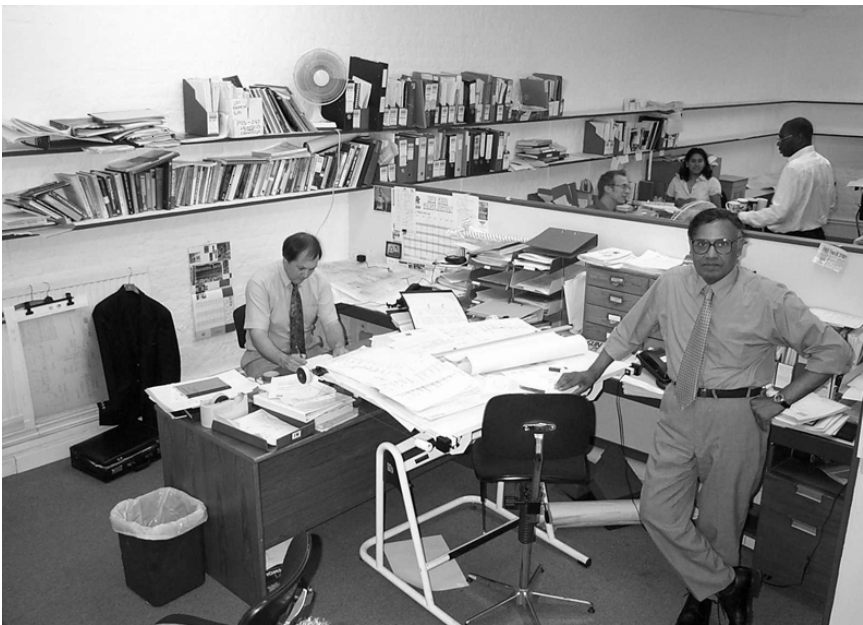
Figure 5.1 What it takes to impose a loading of 2.5 \text{ kN/m}^2 (above); typical office loading of about 0.7 \text{ kN/m}^2 (below).
