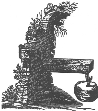
Figure 3.5 Illustration of cantilever from Galileo's A Discourse on Two New Sciences , 1636.
