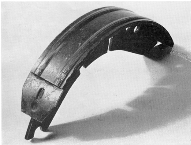
Figure 27.28 Drum brake neglect in service ( Ferodo )
