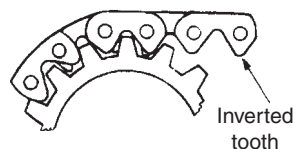
Figure 1.109 Inverted-tooth chain timing drive
