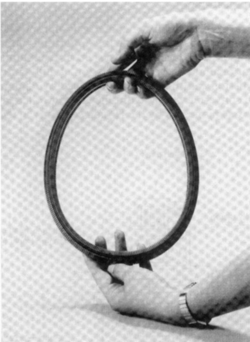
Figure 17.39 High-friction steel thrust belt used in Ford CTX (Ford)
