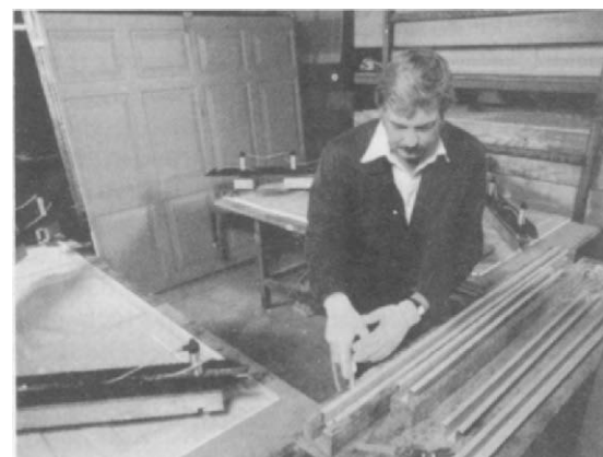
FIGURE 33.14 Mild steel stiffeners are bonded to up and over garage door. Result: rigidity, unblemished exterior surfaces.
