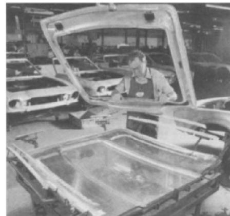
FIGURE 33.13 A structural adhesive used to bond a stiffener to an aluminium car bonnet. To line up the two parts a purpose made fixture is designed.
