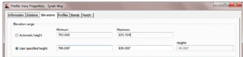
FIGURE 7.66 Modifying the height of the profile view
