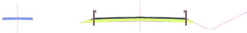
FIGURE 10.68 12' Lane Road With GR And Bikepath assembly with the BasicLane as a bike path
