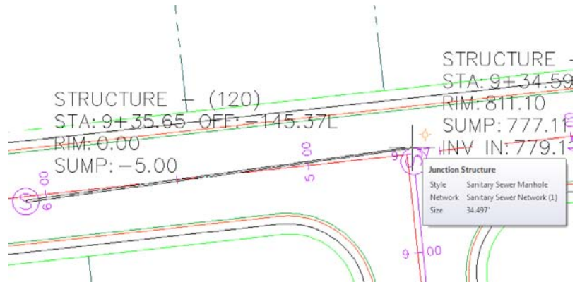
FIGURE 13.37 The connection marker appears when your cursor is near the existing structure.
