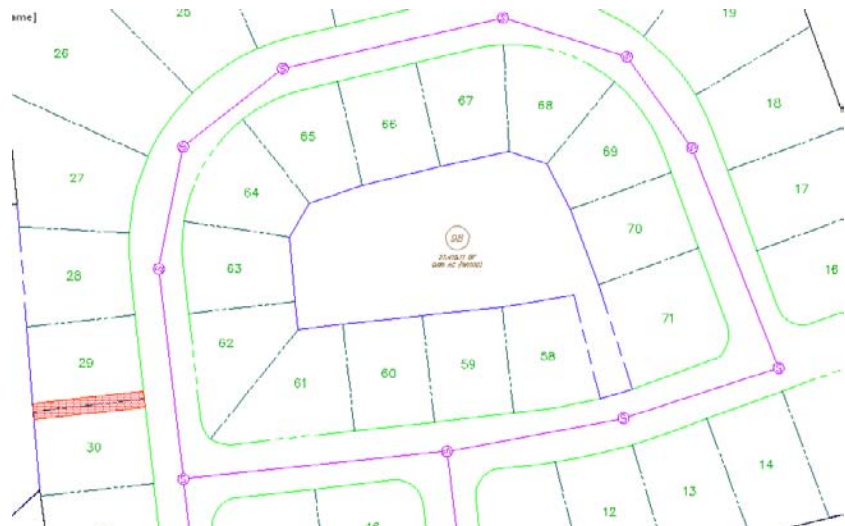
FIGURE 13.24 A typical Civil 3D pipe network
