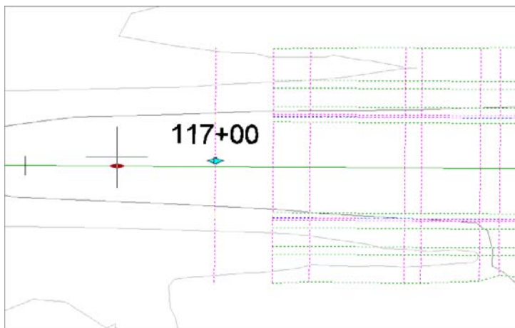
FIGURE 10.38 Change the regions leading up to the intersections using grips (a) or in Corridor Properties (b)
