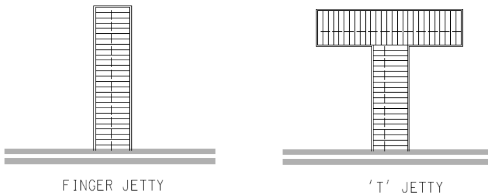
Fig. Finger jetty and T-shaped jetty
