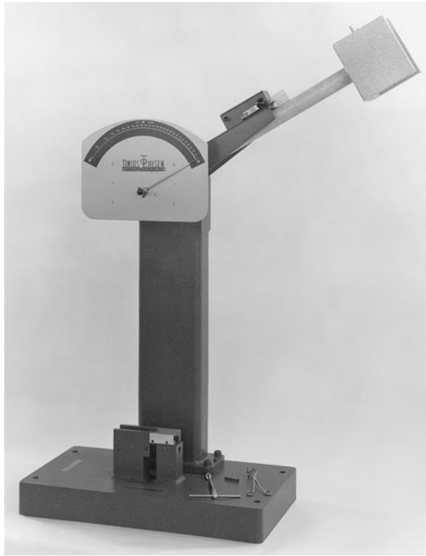
Figure 4.36 Charpy testing machine, shown with the pendulum in the raised position prior to its release to impact a specimen. (Photo courtesy of Tinius Olsen Testing Machine Co., Inc., Willow Grove, PA.)
