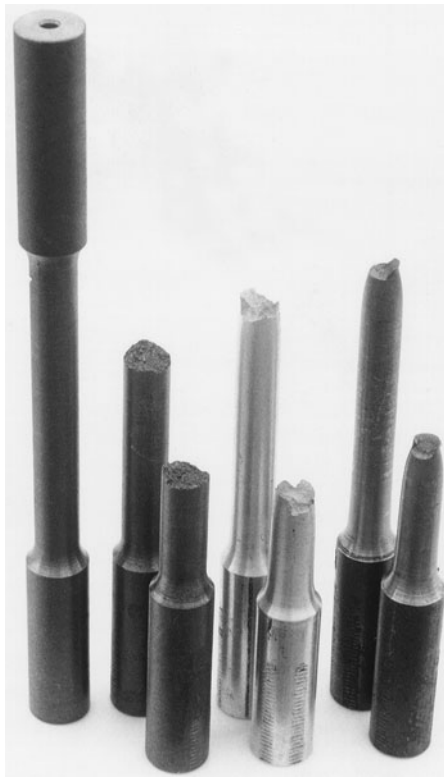
Figure 4.5 Tensile specimens of metals (left to right): untested specimen with 9 mm diameter test section, and broken specimens of gray cast iron, aluminum alloy 7075-T651, and hot-rolled AISI 1020 steel. (Photo by R. A. Simonds.)
