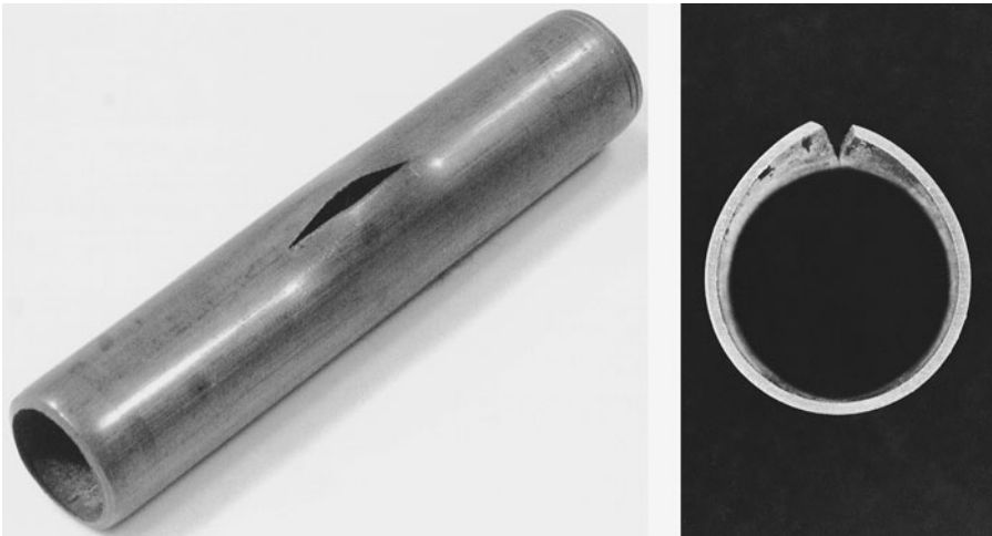
Figure 6.12 Failure of a 15 mm diameter copper water pipe due to excess pressure from freezing. In the cross section on the right, note that failure occurred on a plane inclined 45^\circ to the tube surface, which is the plane of the maximum shear stress. (Photos by R. A. Simonds.)
