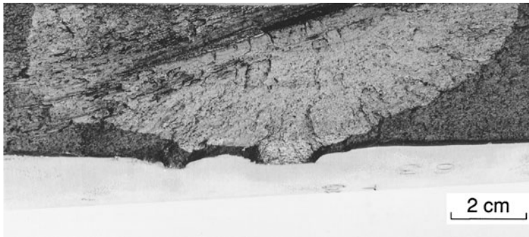
Figure 8.2 Crack (light area) growing from a large nonmetallic inclusion (dark area within) in an AISI 4335 steel artillery tube. The inclusion was found by inspection, and the tube was not used in service, but rather was tested under cyclic loading to study its behavior. (Photo courtesy of J. H. Underwood, U.S. Army Armament RD&E Center, Watervliet, NY.)
