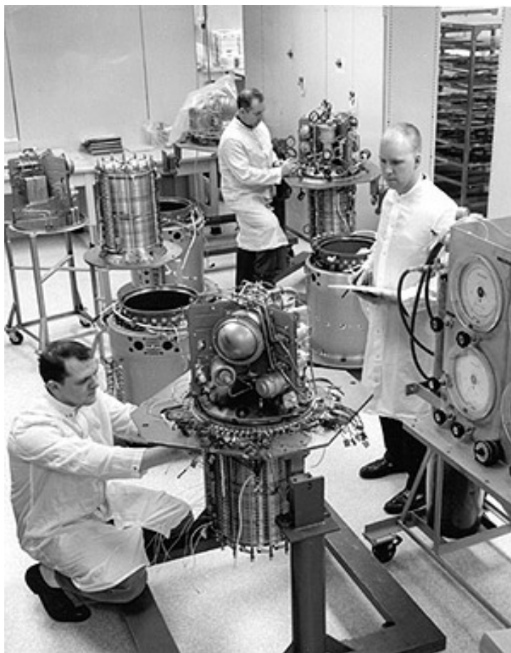
Figure 16 Pratt & Whitney technicians assemble alkali fuel cells for Apollo service modules, 1964. 40
