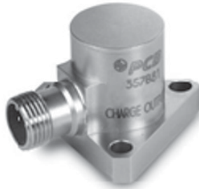
Figure 1.3. Example of piezoelectric accelerometer (PCB 357B81, 2000 g, 20 pC/g, 9kHz shear ceramic) (courtesy of PCB Piezotronics)
