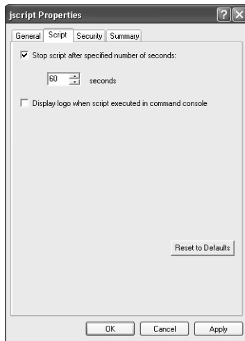
Figure 11-3 You create a WSH file, which contains a script file's settings, by right-clicking the script, clicking Properties, and then clicking the Script tab.
