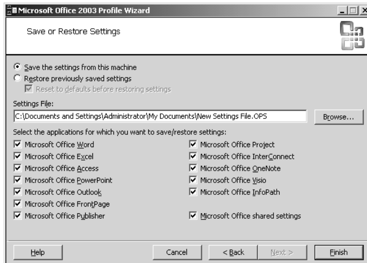
Figure 17-1 The Profile Wizard enables you to exclude settings for some Office 2003 Editions programs and to include settings for others. Clear the check boxes next to the settings that you want to exclude.
