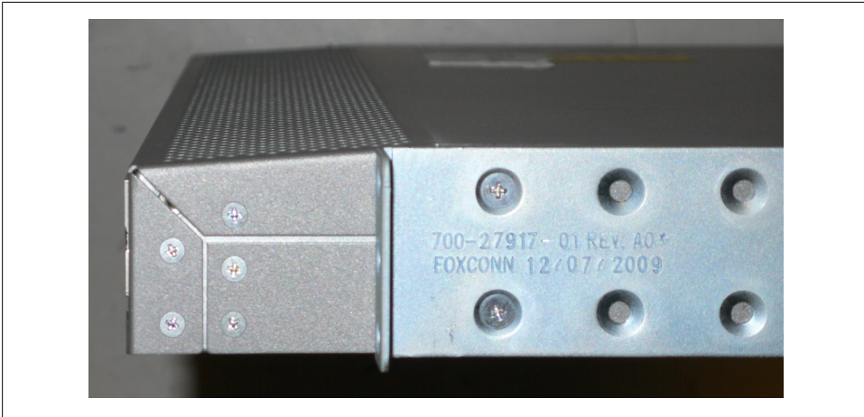
Figure 18-4. A 2148 FEX as seen from the side; notice the airflow vent on top
