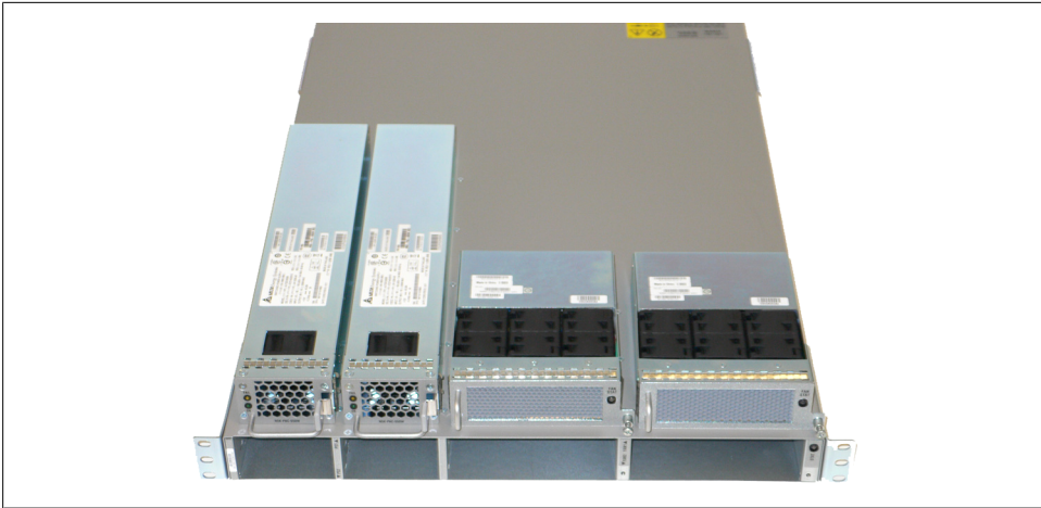
Figure 18-6. Nexus 5010 with power supplies and fan trays removed
