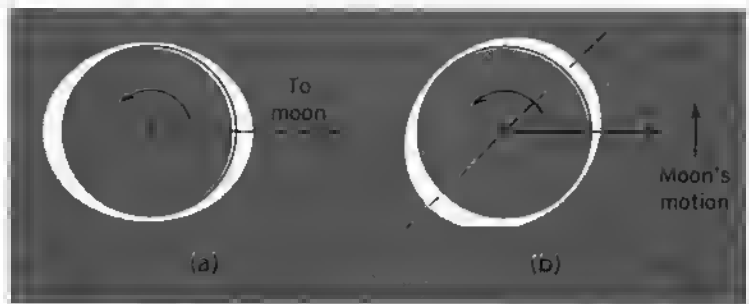
Fig. 12-26 (a) Double tidal bulge as it would be if the earth's rotation did not displace it. The size of the bulge is enormously exaggerated. (b) Approximate true orientation of the tidal bulges, carried eastward by the earth's rotation.
