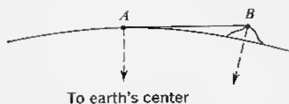
Fig. 6-1 Limitations on inertial motion at the earth's surface. An object starting out horizontally in a truly straight line at A might end up on a hilltop at B. In the process it would be bound to slow down.
