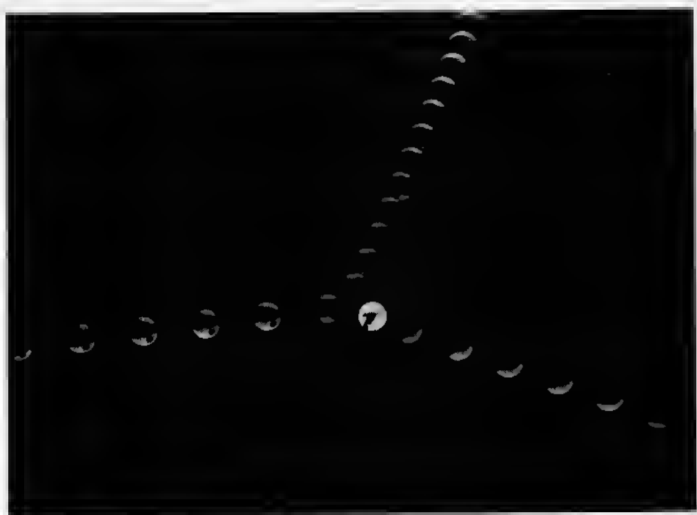
Fig. 9-20 Stroboscopic photograph of an almost perfectly elastic collision between equal masses. (From PSSC Physics, D. C. Heath, Lexington, Massachusetts, 1965.)
