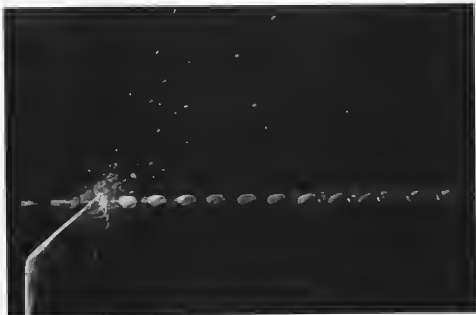
Fig. 6-2 A motion at constant velocity—a bullet traveling at about 1,500 ft/sec, photographed stroboscopically at 30,000 flashes/sec. (Photograph by Prof. Harold E. Edgerton, M.I.T.)
