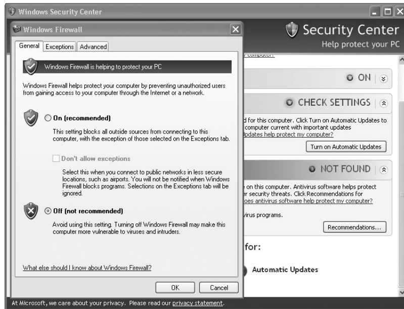
Figure 1-33: Turning off the Windows firewall
