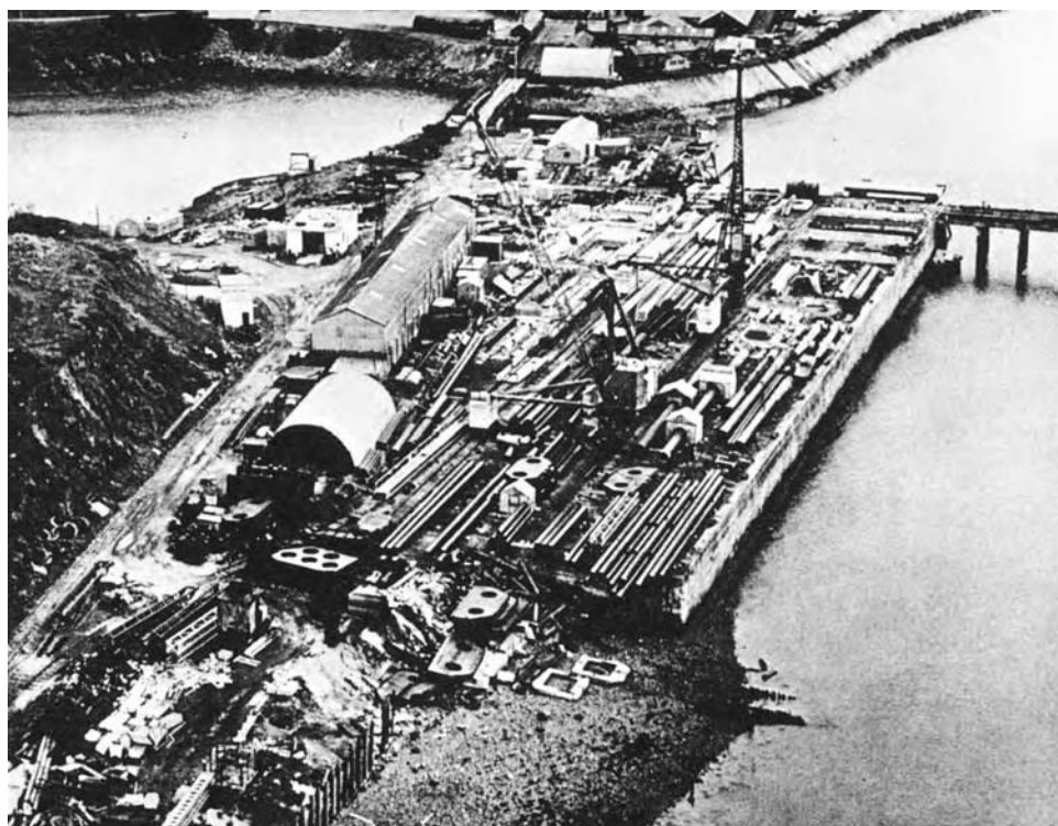
Figure 2.16 Fabrication yard for steel tubular piles at Milford Haven.
