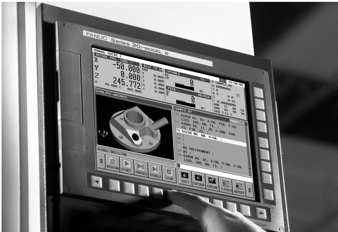
Figure 7-1 FANUC Control Panel Courtesy FANUC FA AMERICA
