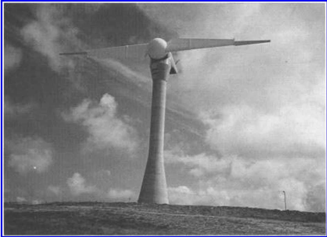
Fig. 5.8. 60 m diameter, 3 MW WT at Burgar Hill, Orkney, by the Wind Energy Group.
