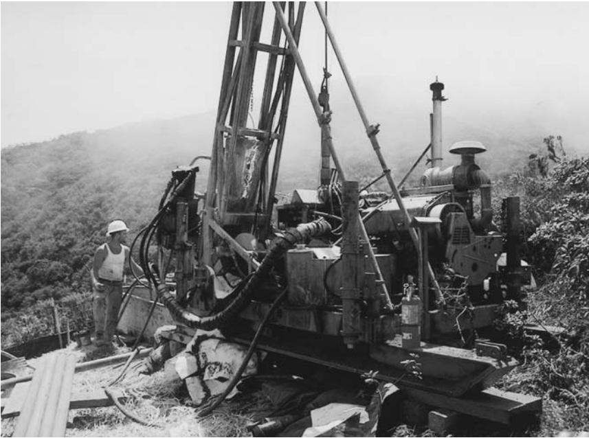
Figure 3.1 Photograph of typical diamond drilling equipment for hole depths up to about 300 m.
