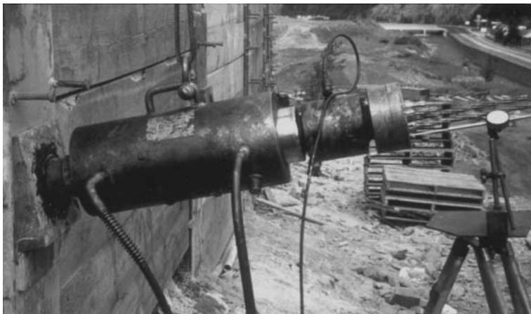
Figure 12.11 Test set-up for a tensioned multi-strand cable anchor comprising hydraulic jack with pressure gauge to measure load, and dial gauge on independent mount to measure anchor elongation. (Photograph by W. Capaul.)
