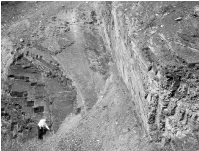
Figure 7.2 Wedge formed by bedding (left) and a conjugate joint set (right); sliding occurred on bedding with joints acting as a release surface (bedded shale, near Helena, Montana).
