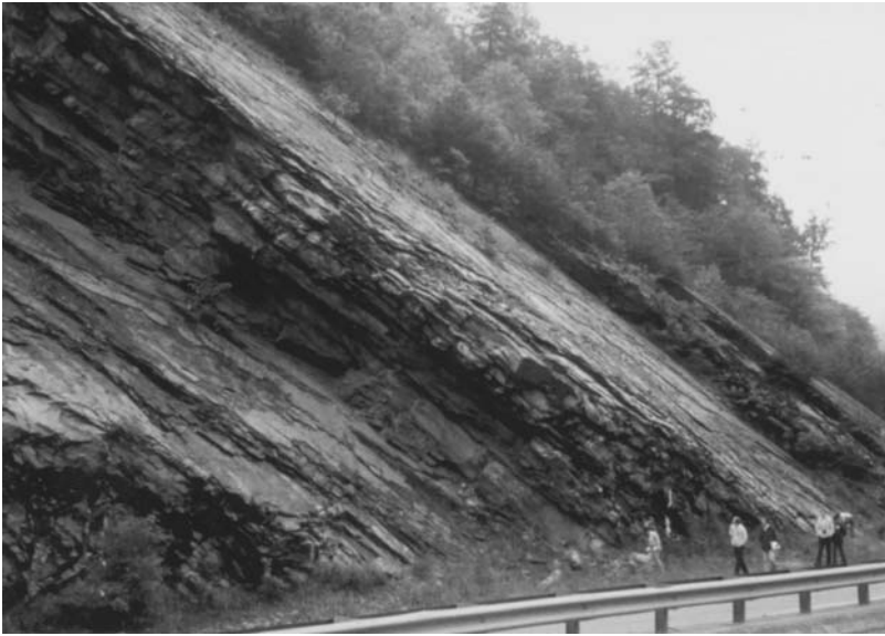
Figure 6.1 Plane failure on smooth, persistent bedding planes in shale (Interstate 40, near Newport, Tennessee).
