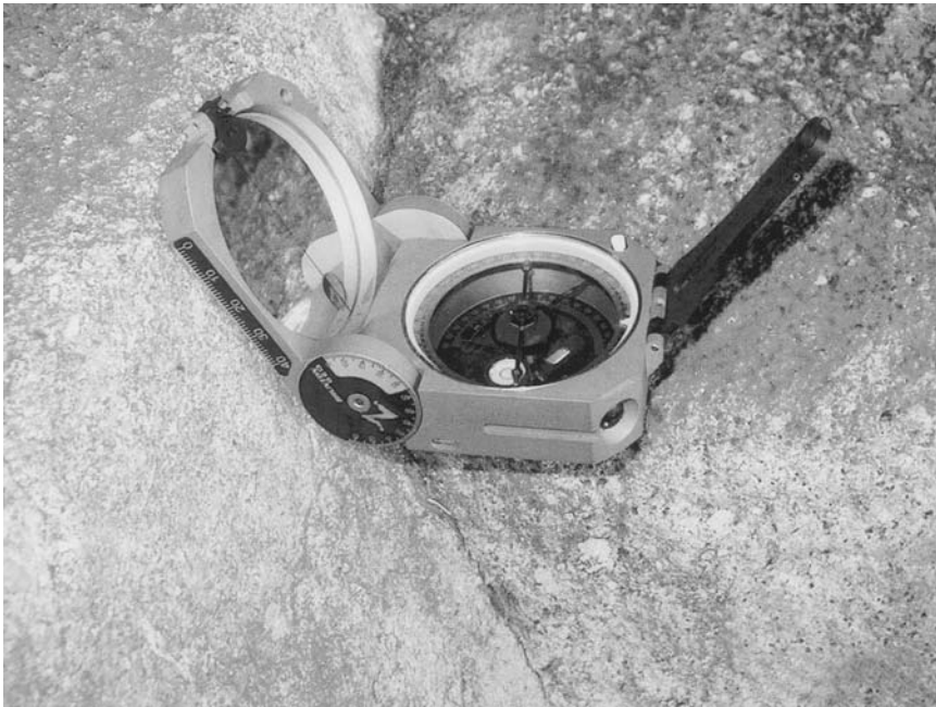
Figure 3.6 Geological compass (Clar type) used to directly measure dip and dip direction of surfaces. Lid is placed on surface and body is rotated until it is level, as indicated by the spirit level; the needle is released to indicate dip direction, and the dip is read off scale on the hinge. (The Brunton Co., Riverton, WY.)
