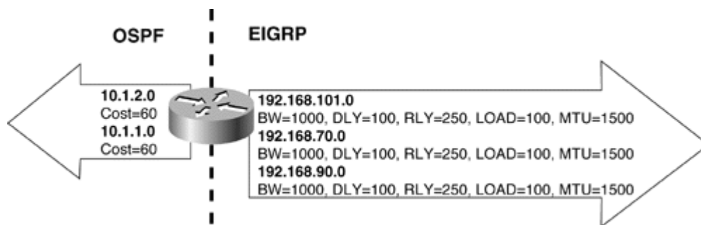
Figure 11.2. When routes are redistributed, a metric that is understandable to the receiving protocol must be assigned to the routes.
