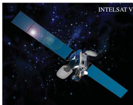
Body Stabilized or Three-Axis Stabilized Satellite (Box Structure)
