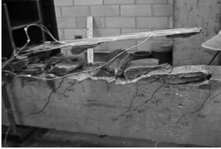
7.12 Fiber optic sensor embedded within the FRP laminate (Zhao et al. , 2007).
