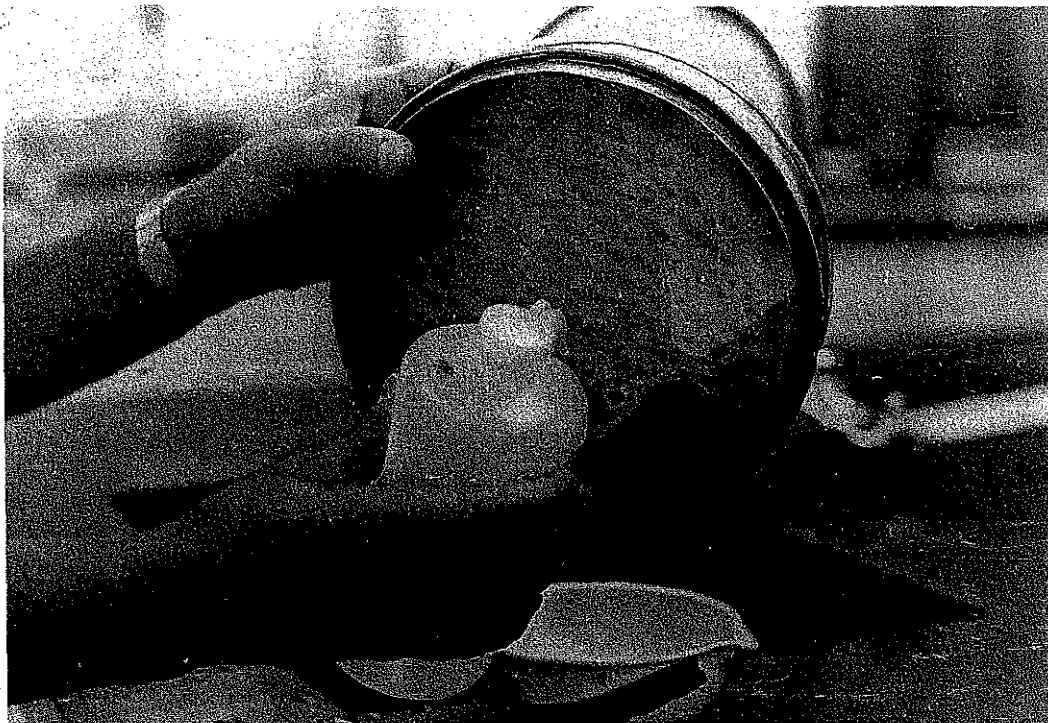
Figure 4-3. Back washing to transfer the soil retained on No. 200 sieve to an evaporating dish.
