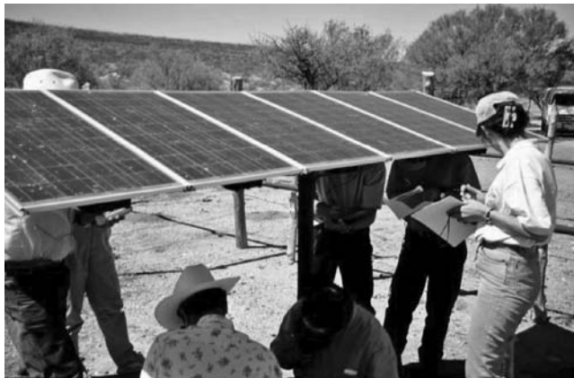
FIGURE 8.44 FIRCO engineers in Mexico learning how to inspect PV water-pumping systems with NMSU and Sandia Labs.
