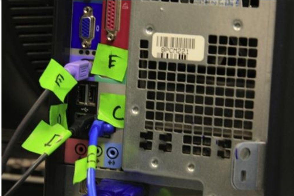
Figure 4.2 Marked cables from the back of a PC. Labels are placed on both ends of a cable to help document how what was connected to the PC at the time it was collected.
