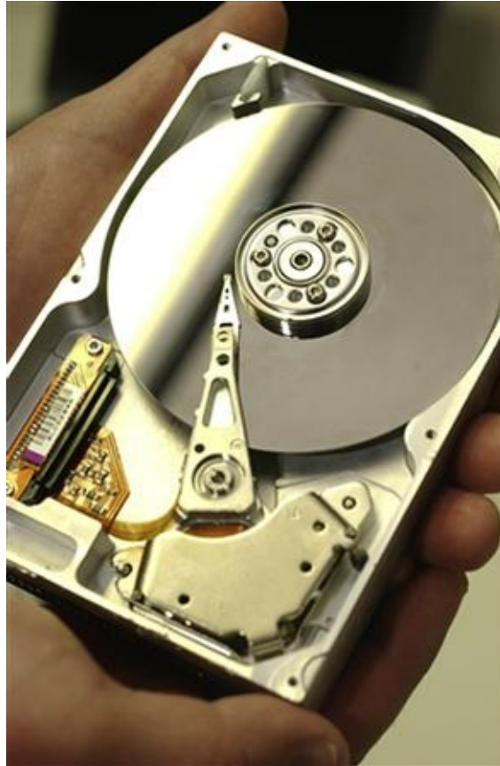
Figure 2.3 The inside of a typical magnetic drive.
