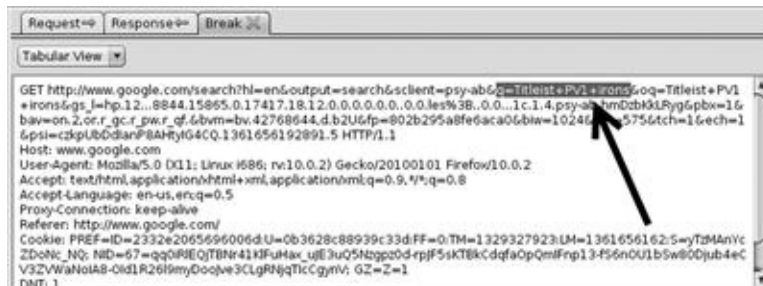
FIGURE 6.16 An intercepted request headed to google.com where the “search” variable is available to be edited.
