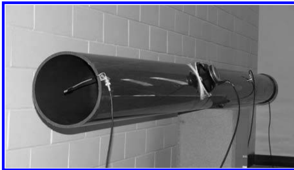
FIGURE 67.2 Acoustic noise in a duct. A noise signal is produced by a loudspeaker placed at one end of the duct. In this photo, a loudspeaker is mounted midway down the duct where it is used to control the noise signal. The pressure at the open end is measured by means of a microphone as shown in the photo. (Photo courtesy of Prof. S. Lipshitz, University of Waterloo.)
