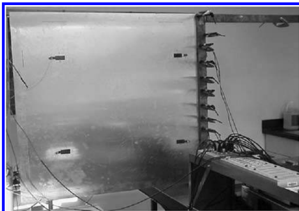
FIGURE 67.3 Vibrations in a plate occur due to various disturbances. In this apparatus the vibrations are controlled via the piezo-electric patches shown. (Photo courtesy of Prof. M. Demetriou, Worcester Polytechnic University.)
