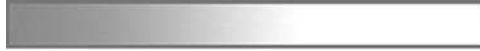
FIGURE 67.4 Heat flow in a rod. The regulation of the temperature profile of a rod is the simplest example of a control system modeled by a PDE.
