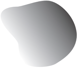
Figure 11.4: The density of a quantity tells us about its distribution over a volume. Where the density is higher, more “stuff” is contained in a part of space. If the density changes in space, we have to integrate the distribution over volume to obtain the amount of the quantity contained in a system.
