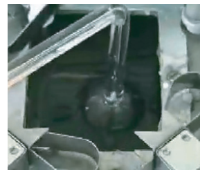
Figure 4.21: Glass bulb containing air serving as an air thermometer. The bulb is in a glycol bath whose temperature can be adjusted. The pressure of the air is measured via the capillary tube visible in the top left corner.
