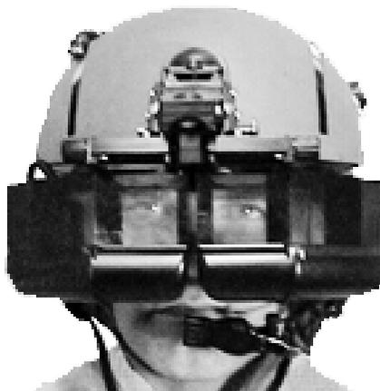
**FIGURE 5.13** Proview™ 100 HMD mounted on SPH-4B helicopter helmet for a simulator application. This is an example of an optically tiled see-through HMD with 100° by 30° field of view. (Photo courtesy of Kaiser Electro-Optics, used with permission.)
