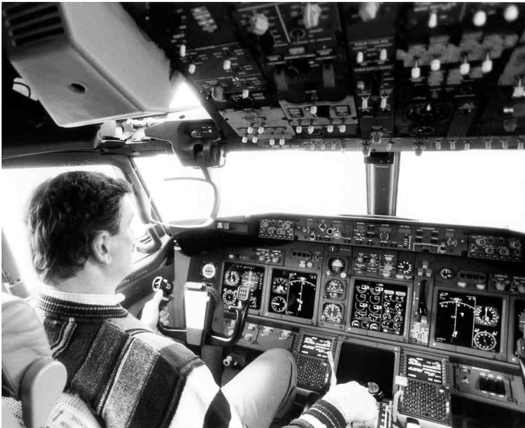
**FIGURE 4.2** Commercial manually flown CAT IIIa HUD installed in a B-737-800.
