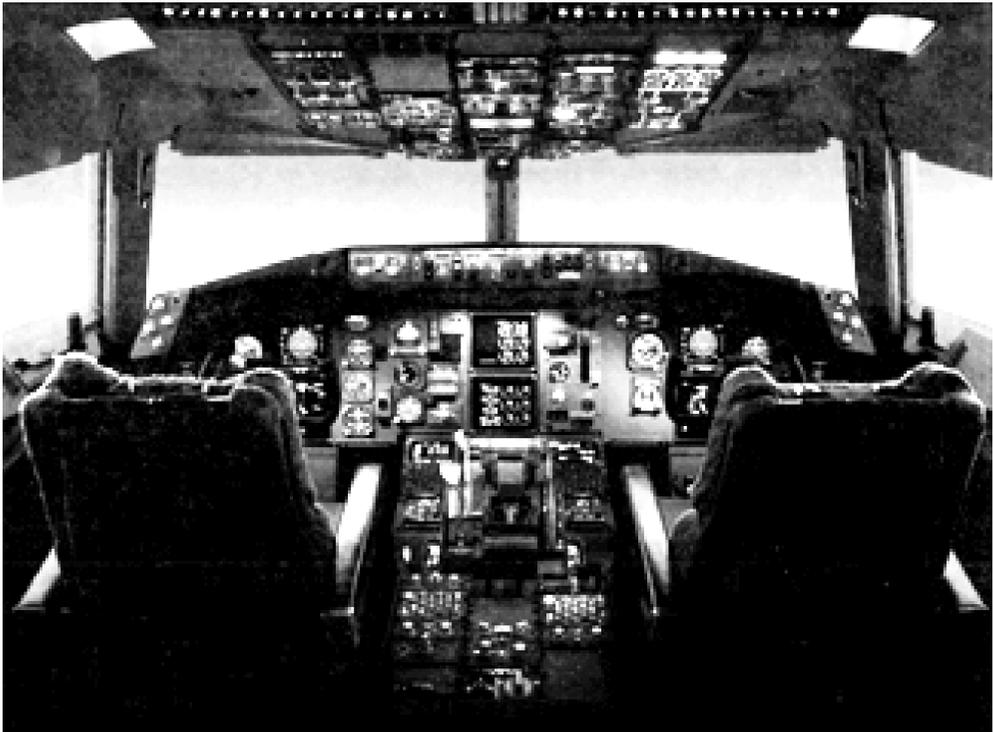
FIGURE 9.3 Representative first-generation “glass cockpit” (B-757) flight deck.
