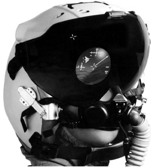
**FIGURE 5.2** The U.S. Air Force and Navy’s Joint Helmet Mounted Cueing System helmet-mounted display that will go into service early in the 21<sup>st</sup> century. (Photo courtesy of Vision Systems International, used with permission.)
