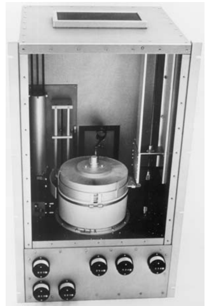
FIGURE 5.85 VHF cavity amplifiers: (a) cross-sectional view of a broadband design, (b) cavity designed for television service, (c) FM broadcast cavity amplifier.
