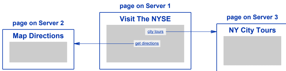
Figure 20.3 An illustration of links in a web page on one web server that reference items on other servers.
