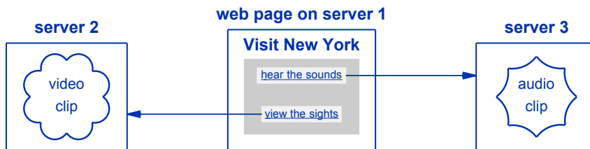
Figure 20.4 Illustration of a web page with links that point to non-text items.
