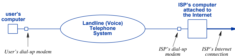
Figure 11.1 Illustration of the equipment used for dial-up Internet access. A modem attached to a user's computer calls a modem at the ISP.
