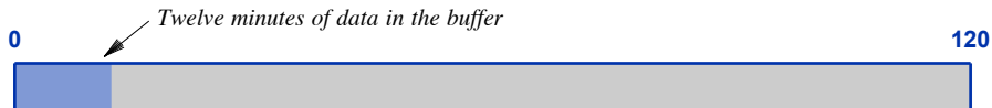
Figure 26.4 An illustration of a playback buffer when it contains the first twelve minutes of a two-hour movie.
