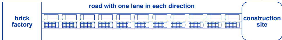
Figure 12.3 Illustration of the road when it is saturated. Trucks are traveling bumper-to-bumper at the speed limit.
