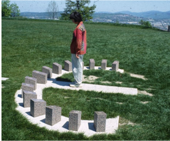
Fig. 1.1 Analemmatic sundial at Saint-Etienne, France in which the user's head forms the gnomon of the dial (Wikipedia 2007)
