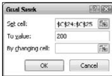
Figure 9.13. Goal Seek finds the input values that give the result you want.
