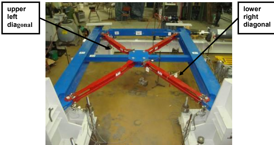
Fig. 4-129 – model H1, graph of the relationship of axial forces N_d against axial displacement (shortening and elongation) of upper left and lower right diagonal (the graph above). A photo showing buckling of upper left diagonal and preservation of the straight form of lower right diagonal (below).
