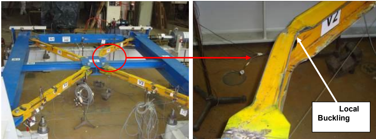
Fig. 4-91 – model H2, axial forces N_d in the diagonals depending on the horizontal force F in cycle 19. In this cycle is registered LB (photos below, right). Behavior of CBF in applied displacement \approx 4,1\Delta_y ;
