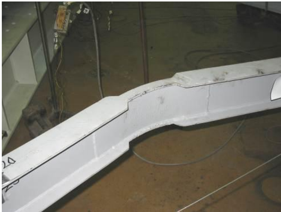
Fig. 4-147 – model H3, middle modified cross section, plastic deformations, no LB
