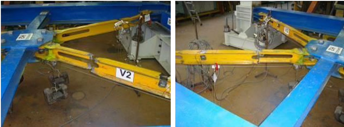
Fig. 4-107 – model H2, forms of fracture of the tensioned diagonals; The photo on the left - upper right diagonal, the photo on the right - bottom right diagonal.
