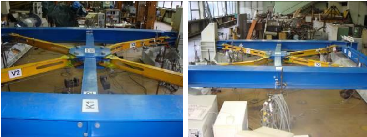
Fig. 4-101 – model H2, bending of the horizontal intermediate member due to unbalanced vertical force;
