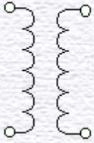
air core for use above 1MHz
