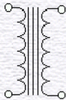
iron core for use at audio & mains frequencies
