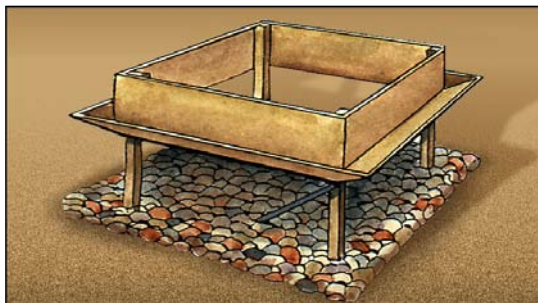
Figure 6.17. Variation of Basic Trough Urinal.
