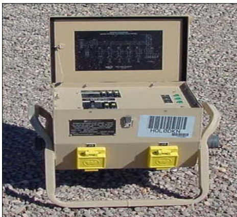
Figure 9.5. Power Distribution Panel (PDP).
