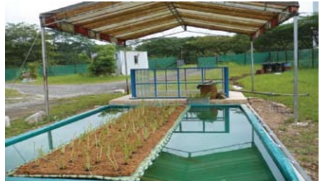
Figure 7. Experimental setup - The Perspex tank
