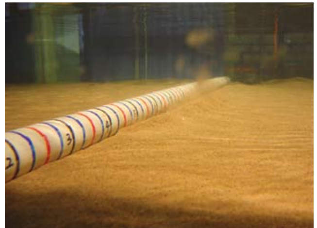
Figure 8. Scour under pipelines in current
