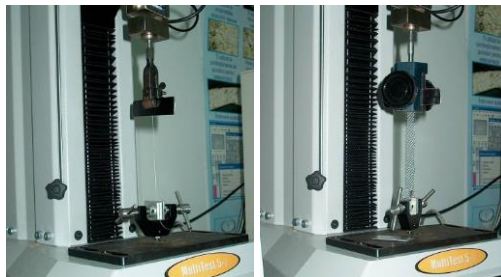
Figure 5. Tensile tests on individual steel wire and steel meshes
