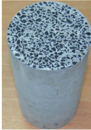
Figure 1. Cylinders made of concrete and rubber
