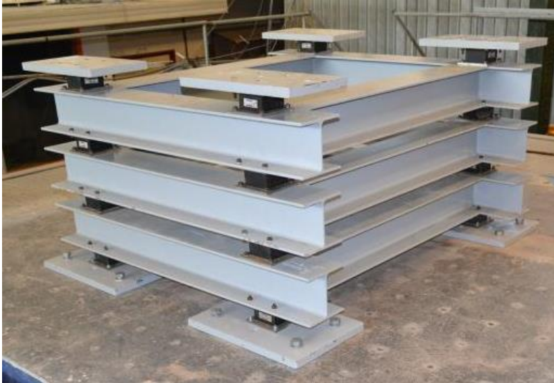
Figure 2. Multi-stage isolation system with elastomeric bearings
