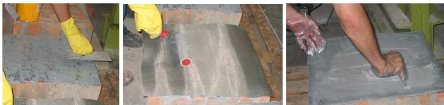
Figure 1. Retrofitting solution based on epoxy-glued steel wire mesh (SWM)
