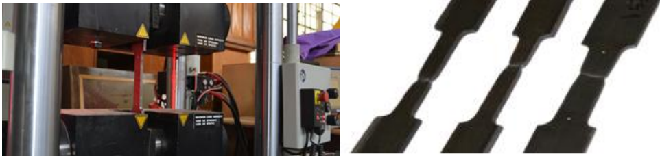
Figure 3. Tensile test in progress (left); coupons with monitored white dots (right)
