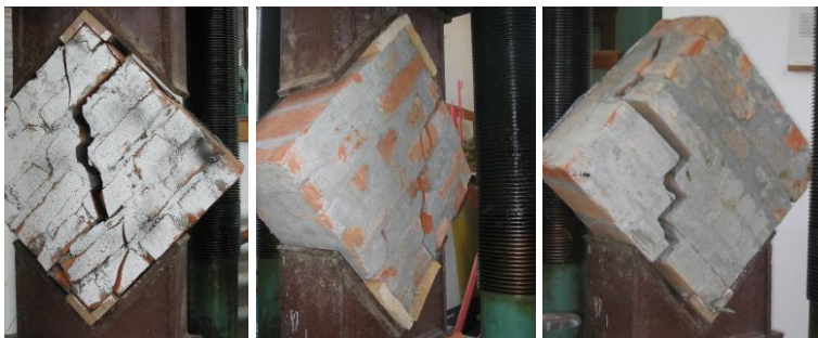
Figure 9. Damage pattern of one side retrofitted elements with swm
